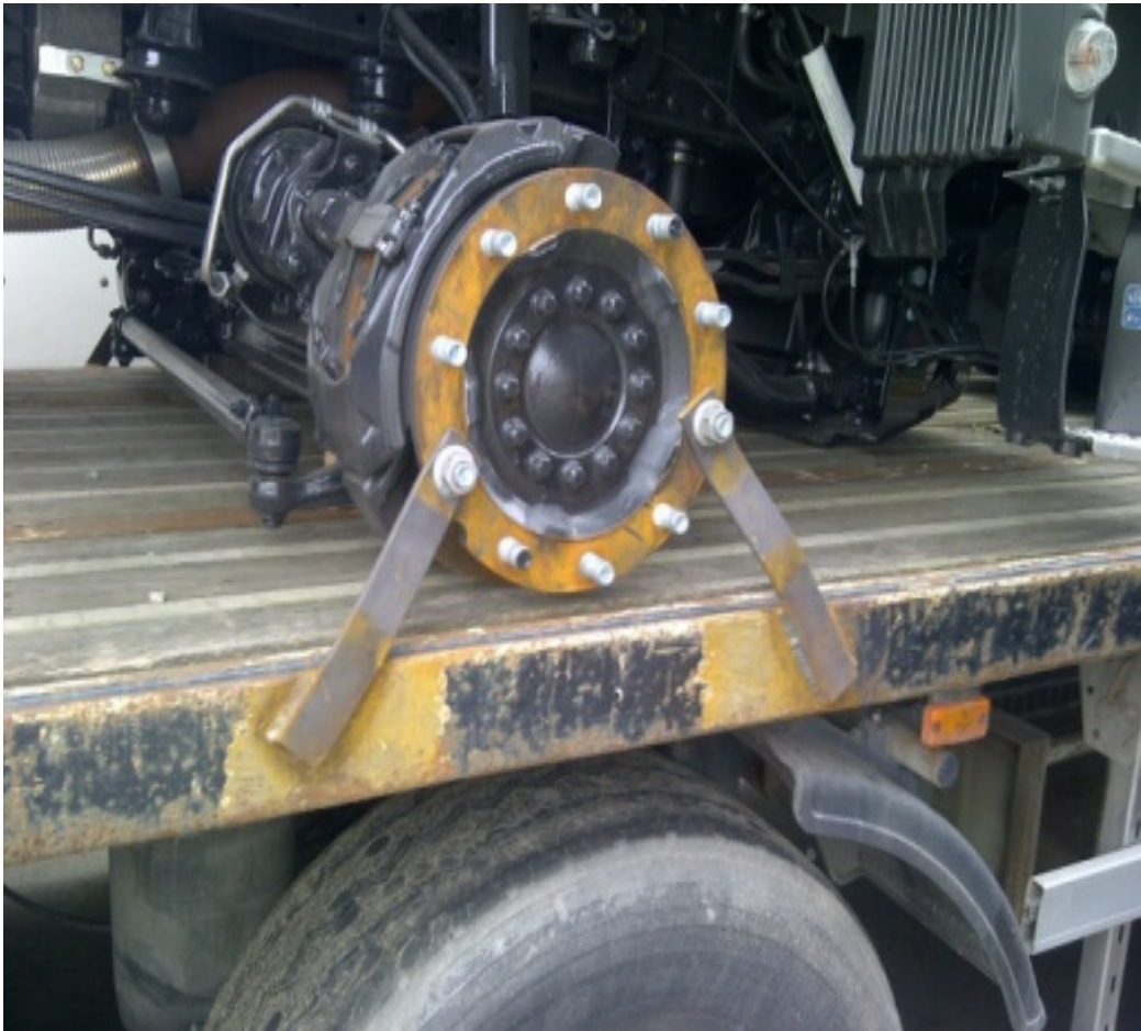
Acceptable welded lashings directly onto axle disks – metal bars are bolted to axle disk
