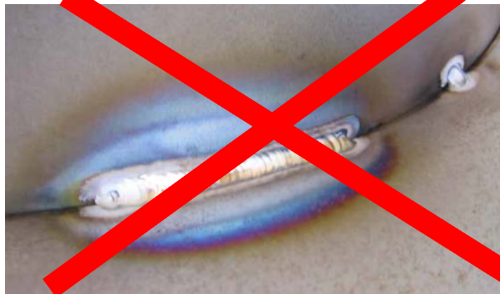
Do not weld Bonnets shut
